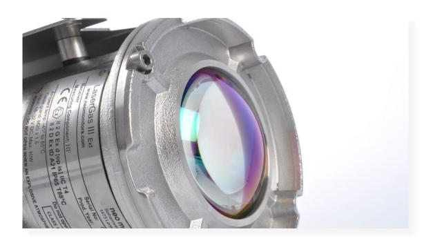
NEO Monitors LaserGas™ III Open Path Gas Detector is based on our highly successful LaserGas™ III platform and is specifically designed for measurements in critical emission monitoring and fence line applications in hazardous areas. Utilizing separate compact Exd flameproof enclosures, the transmitter and receiver units can be mounted up to 100 meters apart (application dependent), allowing gas concentration measurements along the optical path to be detected in real-time.
