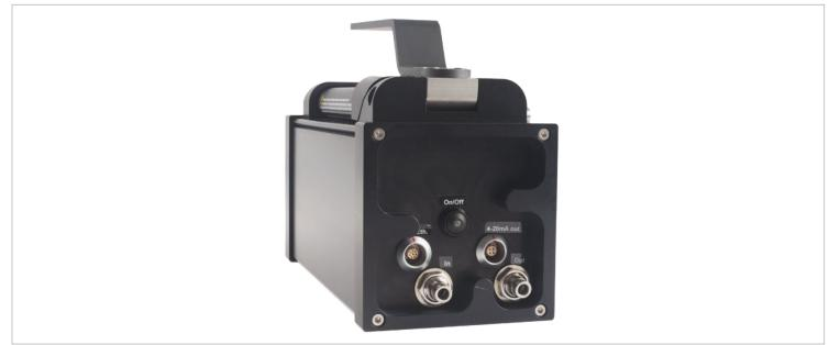
NEO Monitors LaserGas<sup>™</sup> is using Tunable Diode Laser Absorption Spectroscopy (TDLAS) i.e. a non-contact optical measurement method employing solid-state laser sources. The portable analyzer is compact, lightweight, and battery powered for HF measurement on the spot. With onboard pump and connections for Teflon tubing the target gas is continuously transferred into the internal measurement cell. The instrument´s low power design gives long operating time on each battery cycle.
